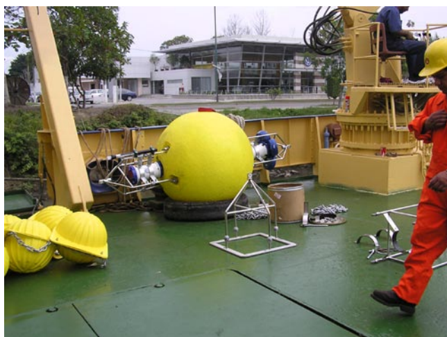
On board R/V Justo Sierra : 300 kHz Workhorse and 75 kHz Long Ranger mounted on the upper float
